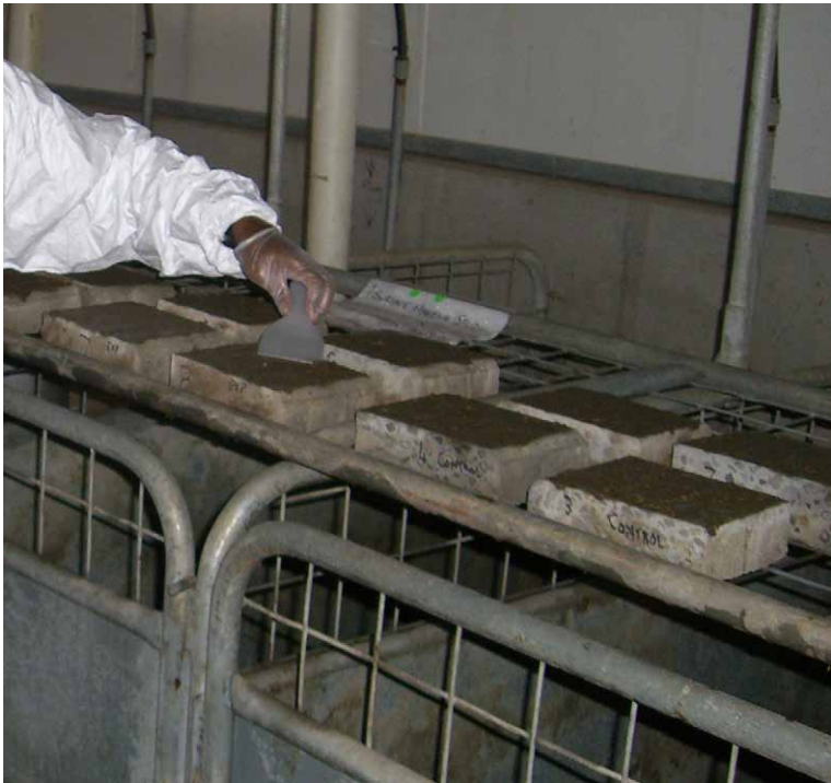
Figure 18.2. Application of pig manure on experimental pavers.
