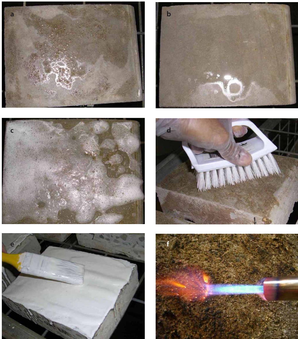
Figure 18.5. Various cleaning methods applied to soiled floor pavers. (a) hosing; (b) pressure washing; (c) degreasing; (d) dry scrubbing with wire brush; (e) liming using builder's lime; and (f) flaming.
