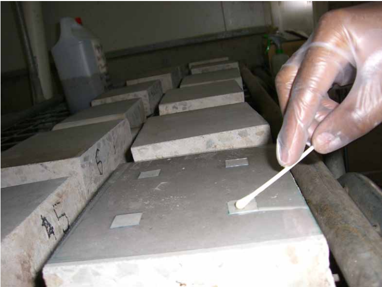
Figure 18.4. Taking swab samples from hygiene pavers.
