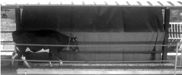
Figure 22.2. Side view of a cow walking over the measurement zone for gait scoring; the pressure sensitive mat is inside the measurement bridge. An automatic gate and antenna for cow identification is located at the entrance of the measurement zone (not shown).
